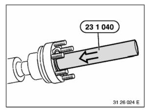
Drive constant-velocity joint onto propeller shaft using Special Tool 23 1 040.
