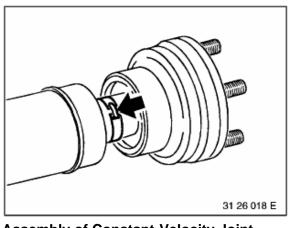
**Assembly of Constant-Velocity Joint**
