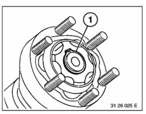
Install circlip (1).
