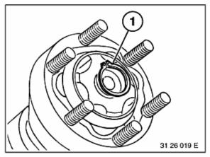
Lift out circlip (1).
