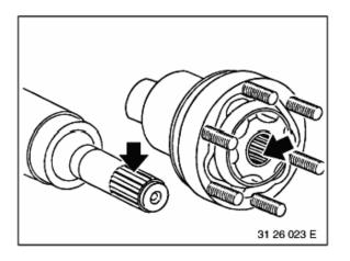
Clean splines to free them of grease and coat with bolt cement (refer to BMW Parts Service).
